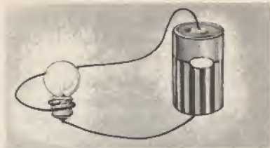
No current flows in the circuit (above left), because there is no "electron pump"—no source of power. Current flows in the circuit (above right), because the dry cell acts as electron pump.
